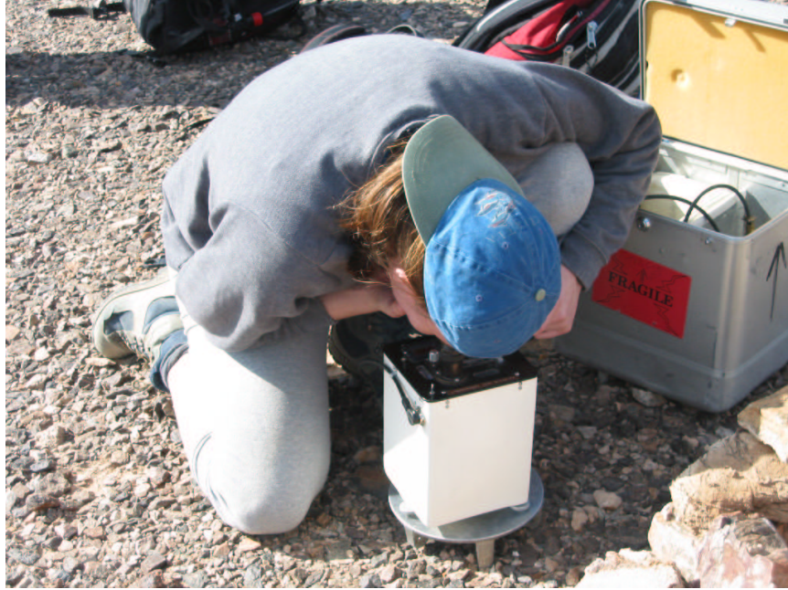
Figure 13: Typical position for the gravimeter operator
