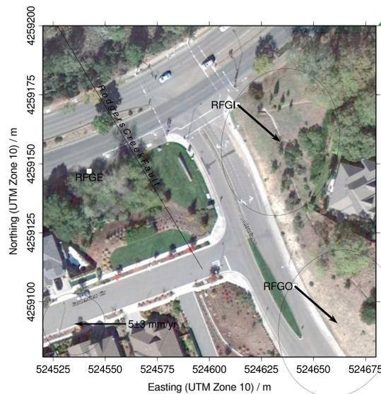
Figure 2: Zoomed view of current GPS velocities at alignment array 'RCFG' (Rodgers Creek: Fountain Grove Parkway), relative to site RFGE. Though these velocities are based on just one year of data, further measurements may support the existence of surface creep.
