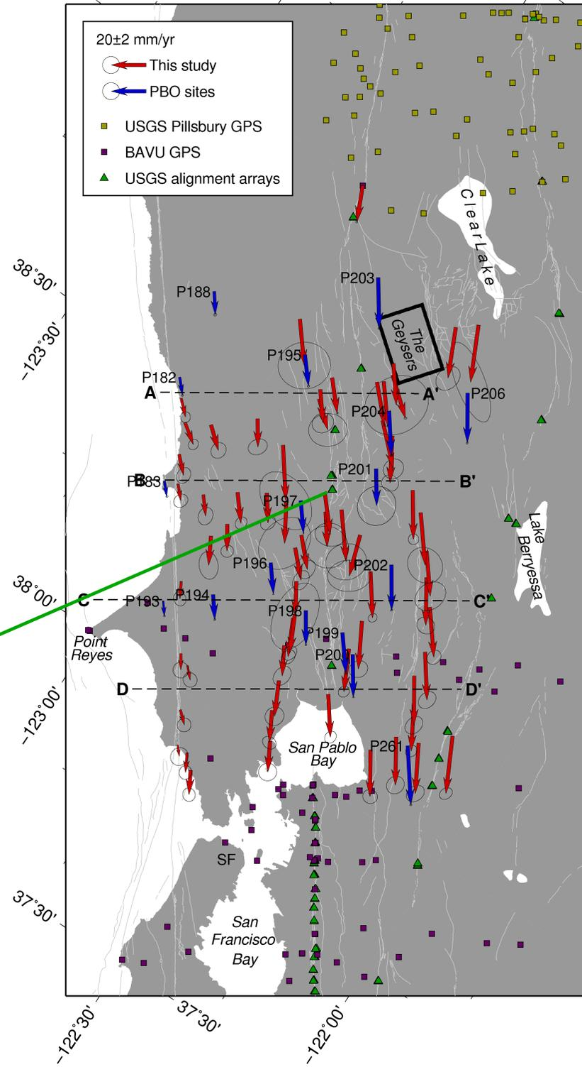
Figure 1: Velocity solution relative to Pacific plate (ITRF2005, Altamimi et al, 2007). Only sites whose 1-sigma uncertainties are less than 10 mm/yr are shown here. More sites have been occupied, especially near Santa Rosa (intersection of Rodgers Creek Fault and profile B-B'), but currently suffer from a lack of observation period ( $\leq 2$  years).
