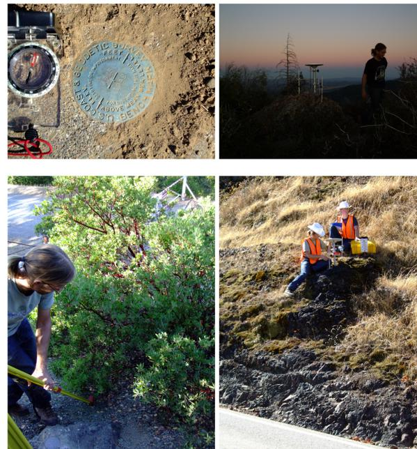
**Figure 2:** Top-left Existing marks, ideally plated by the US Geological Survey or National Geodetic Survey (formerly US Coast & Geodetic Survey) are sought to measure. Top-right Brad walks away from a new overnight occupation of site DIVD in The Geysers area in September 2009. Bottom-left Brad secures the tripod among shrubs. Bottom-right Gareth and Brad defy the slopes to occupy a mark above the road.
