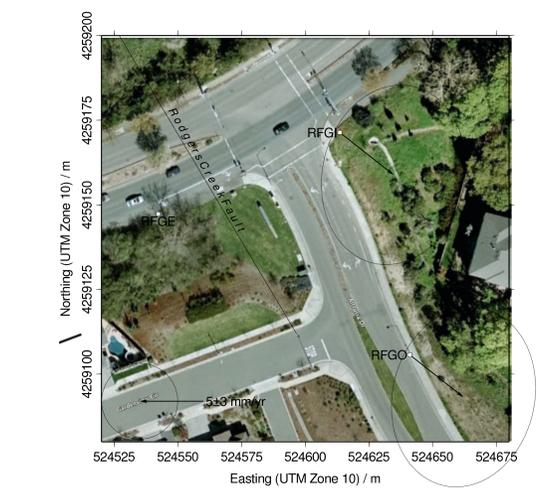
**Figure 5:** Zoomed view of the alignment array at Fountain Grove Parkway, Santa Rosa. Sites RFG1 and RFGO have equated velocities which are shown with respect to RFGE, on the south-west side of the fault. Ground imagery courtesy of Google Earth and the City of Santa Rosa.
