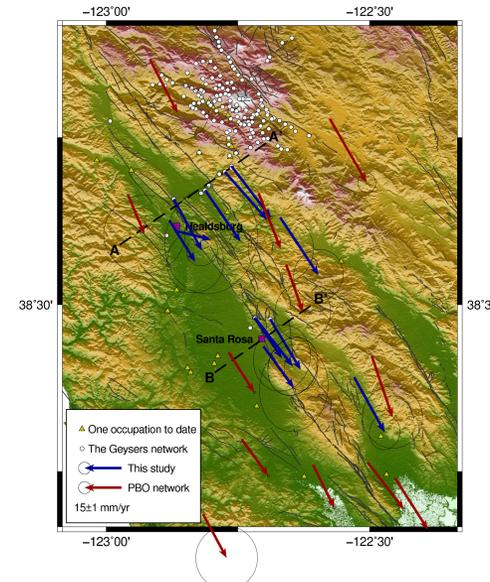
**Figure 3:** Velocity solution obtained in this work to date. Only 13 sites that are not included in The Geysers network have been occupied more than once (blue velocity vectors). White dots indicate GPS sites measured by Mossop and Segall (1997) and Gettings *et al.* (2002), combined. These velocity data are vital to the problem to be solved here as deformation in The Geysers heavily dominates and overprints any fault-related strain on the north-east side of the Maacama Fault.
