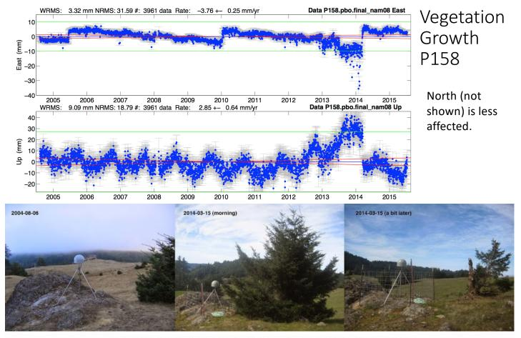
Figure 4. P158 at installation (left), ~10 years later (middle), ~10 years+2 hours later (right). The small tree north of the station grew into a larger tree and was removed on March 3, 2014. Earthquakes and non-linear motions
