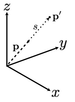
$$\mathbf{p}' = \mathbf{p} + s\mathbf{p} \ egin{pmatrix} p_x' \ p_y' \ p_y' \ p_z' \end{pmatrix} = egin{pmatrix} p_x \ p_y \ p_z \end{pmatrix} + s egin{pmatrix} p_x \ p_y \ p_z \end{pmatrix}$$
