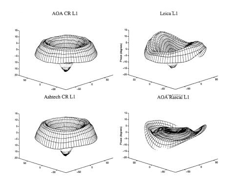
*Left:* Examples of the antenna phase patterns determined in an anechoic chamber...BUT the actual pattern in the field is affected by the antenna mount
