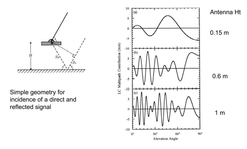
Multipath contributions to observed phase for three different antenna heights [From *Elosegui et al*, 1995]
