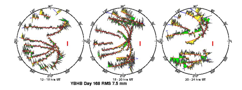
One-way (undifferenced) LC phase residuals projected onto the sky in 4-hr snapshots. Spatially repeatable noise is multipath; time-varying noise is water vapor.
