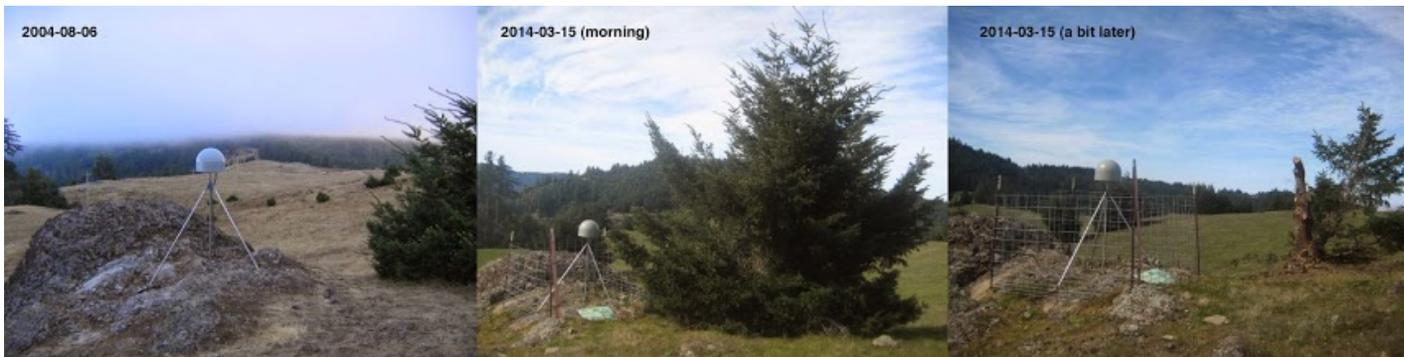
Figure 4. P158 at installation (left), ~10 years later (middle), ~10 years+2 hours later (right). The small tree north of the station grew into a larger tree and was removed on March 3, 2014.
