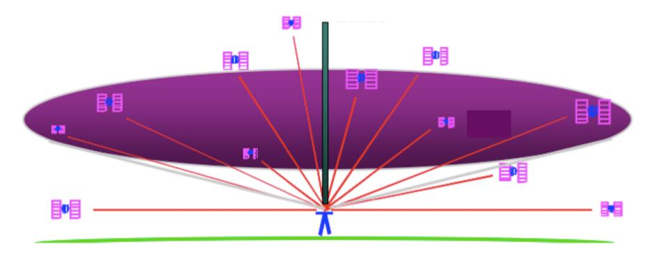
The signal from each GPS satellite is delayed by an amount dependent on the pressure and humidity and its elevation above the horizon. We invert the measurements to estimate the average delay at the zenith (green bar).
