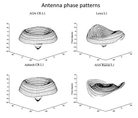
Left: Examples of the antenna phase patterns determined in an anechoic chamber...BUT the actual pattern in the field is affected by the antenna mount
