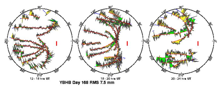
One-way (undifferenced) LC phase residuals projected onto the sky in 4-hr snapshots. Spatially repeatable noise is multipath; time-varying noise is water vapor.
