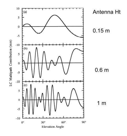
Multipath contributions to observed phase for three different antenna heights [From *Elosegui et al*, 1995]
